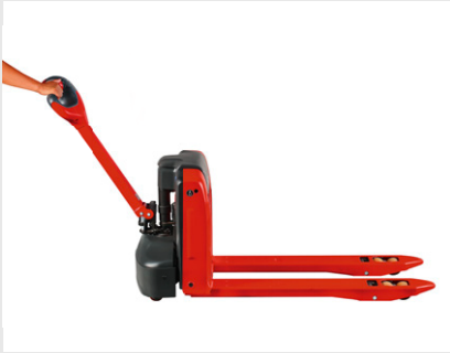
Long low mounted tiller ensures safety distance
